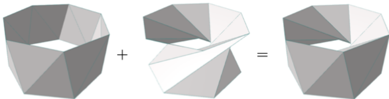
Figure 8: The union of two proids with common bounding polygons is a “diploid torus” or “diploitor”.
